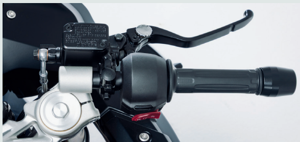
Ride-by-wire throttle with 4 riding modes
