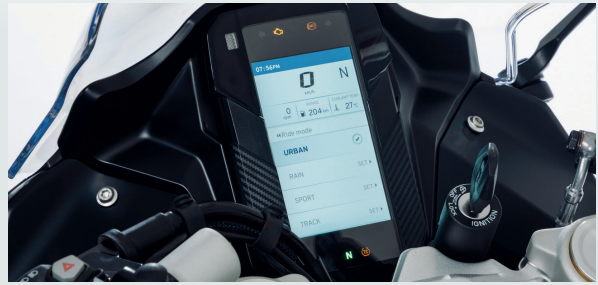
5" TFT Race Computer with SmartXconnect connectivity, delivering navigation and real-time ride data
